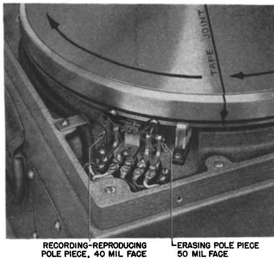
FIG. 10. View with cover removed, showing the magnetic tape and the pole pieces. The butt joint in the tape is exaggerated in this picture.
